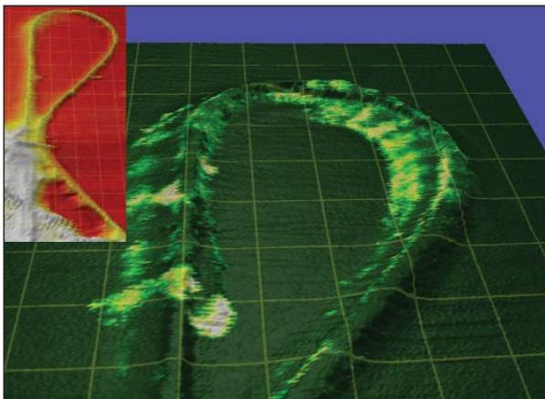
At first glance, the image could be a three-dimensional map of a pier jutting off a coastline, or some strange earthwork. But it is on an entirely different scale: a carbon nanotube, resting on a silicon dioxide surface, next to a smattering of gold atoms.
