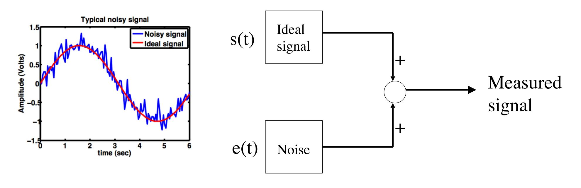
By making assumptions about the properties of the unwanted 'noise' e(t), we can reconstruct an appropriate estimate of the original signal
