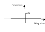
Static Friction Model: Friction force opposes the direction of motion when the sliding velocity is zero.
