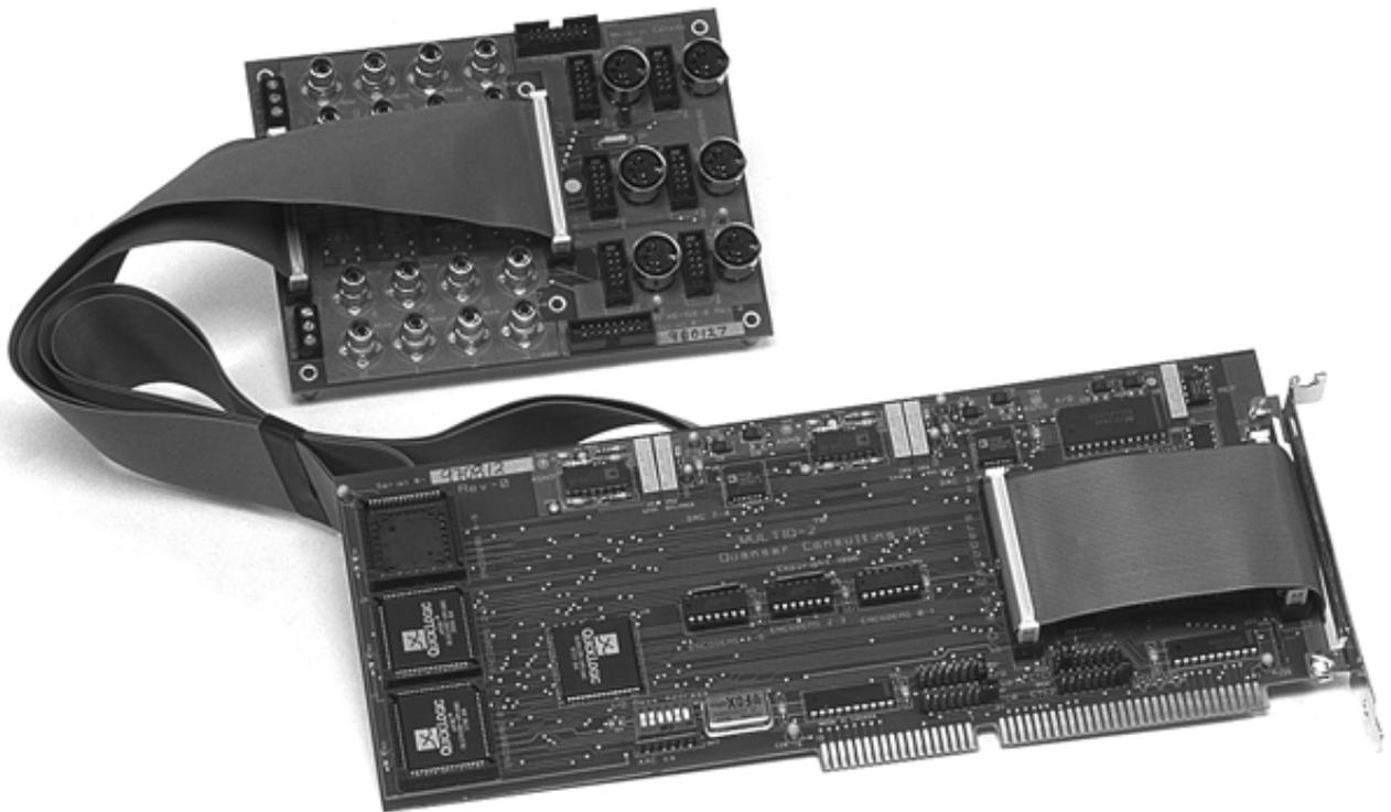
*Photo of MultiQ-2. The MultiQ-3 has 8 encoder connectors on the terminal board.*
